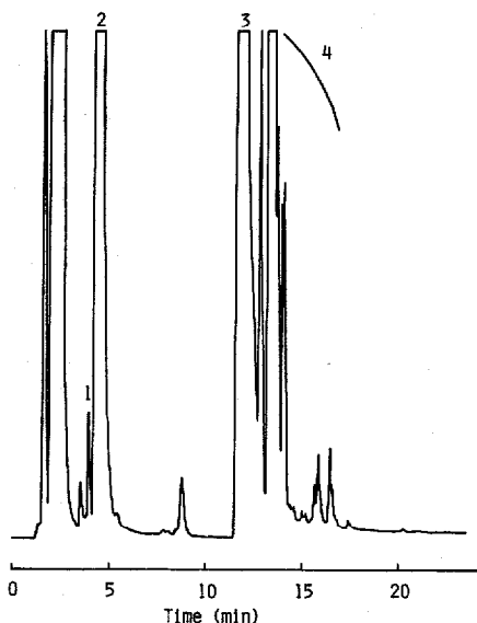
Fig. 5. Typical chromatogram of Zpt adsorbed on human hairs. 1, Zpt (compound III); 2, compound IV; 3, N-dansylaziridine; 4, unknown.
